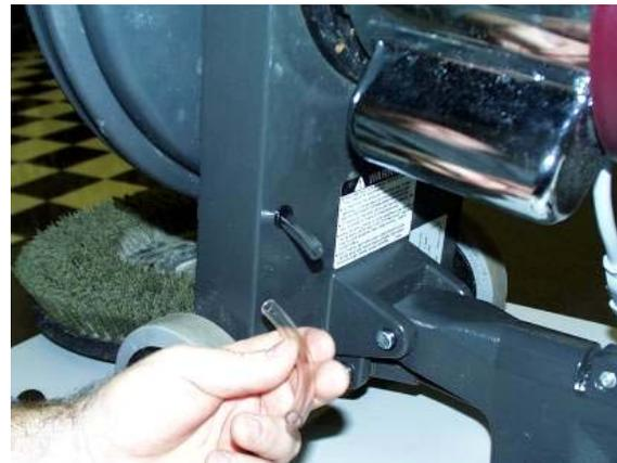
Slide the plastic sleeve onto the tube and into the hole (as shown above). Then trim the HOSE-1/4 ID X 8" LONG (**190423**) so that there is about 1-1/2" of tubing protruding from the frame.
