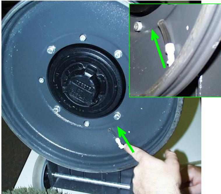
Install the tube assembly into the hole in the bottom of the housing (oriented toward the center hub) as shown above.
